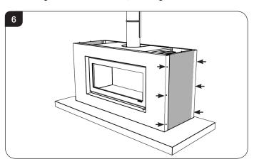
2.6 Position the Top Panel carefully without the Rear Slider Panel and press into place see Diagram 7.
